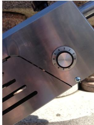
5. With *small changes only* adjust the propane dial when the propane has ignited and you see steam flowing from the end of the Gumwand after 5 – 10 seconds.
