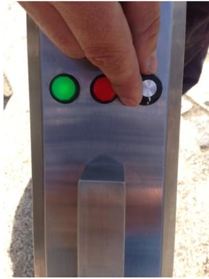
3. Push the red ignition button. This will start the internal ignition procedure:
