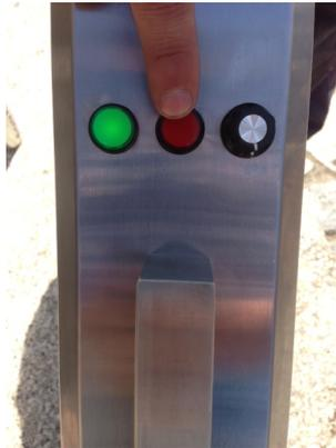
4. Slowly turn the Propane dial up until the Propane ignites in the burner. You will hear the propane ignite. If the sparking from step 3 stops, you will hear a beeping alarm to indicate there is no Propane detected. Press the red button again to start the sparking action
